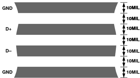
Figure 19. Arrangement of Signal Tracks
